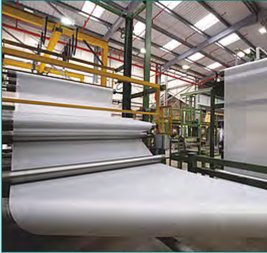
VINYL FLOORING IN PRODUCTION PHOTO : POLYFLOR LTD
