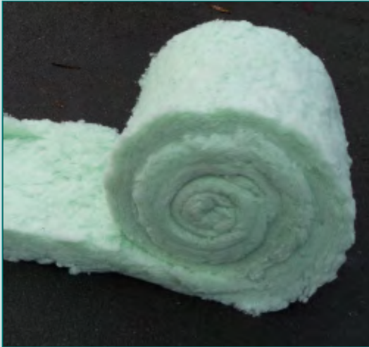
RECYCLED PLASTIC BOTTLE INSULATION PHOTO: JO DENISON, STEPHEN GEORGE + PARTNERS
