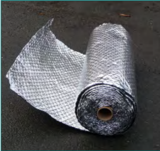
MULTIFOIL INSULATION PHOTO: JO DENISON, STEPHEN GEORGE + PARTNERS
