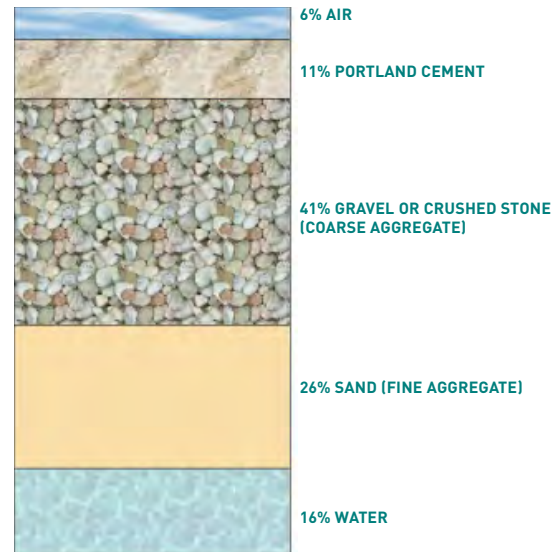
THE COMPOSITION OF CONCRETE
